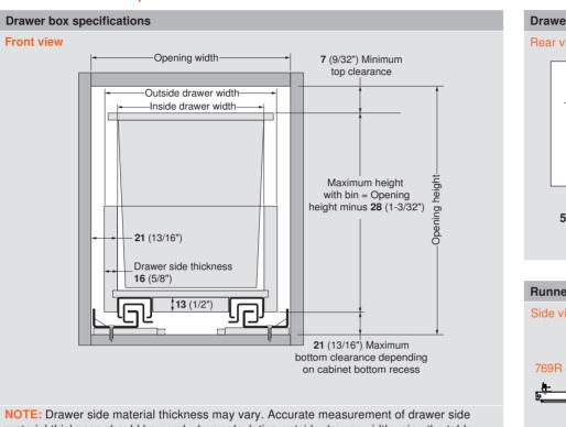
**NOTE:** Drawer side material thickness may vary. Accurate measurement of drawer side material thickness should be used when calculating outside drawer width using the table below. Inside drawer width **must** equal opening width minus **42** (1-21/32") for MOVENTO runners to align and function optimally.
