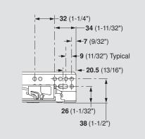
NOTE: Elongated holes are for ±4.5 (3/16") depth adjustment only. Additional screws must be used to secure the runner to the
